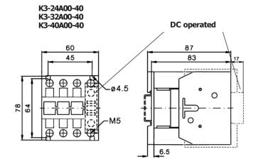
Contactors 4-pole, AC operated / DC operated
